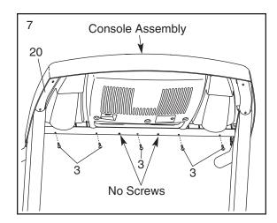
8. Hand tighten four additional Screws (3) into the Handrail (20) and the console assembly. Then, tighten all nine Screws used in step 7 and this step; do not overtighten the Screws.
